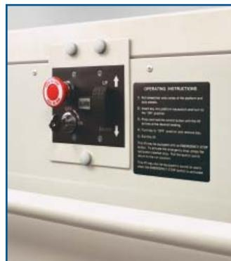
Standard controls on the lifts include a constant-pressure directional paddle, an emergency stop button, illuminated alarm button, and a key lock to secure against unauthorized access.
